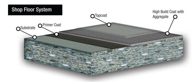
Shop Floor System is a high build, colored epoxy/urethane, high performance concrete coating system. It is used for environments requiring an attractive, high performance floor or when a concrete floor has sustained damage requiring a moderately thick surfacer with a slip resistant texture.
